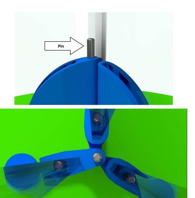
Then for the outer brace using a screw so that it can be used for tables of various thicknesses, a maximum of 40 mm.
