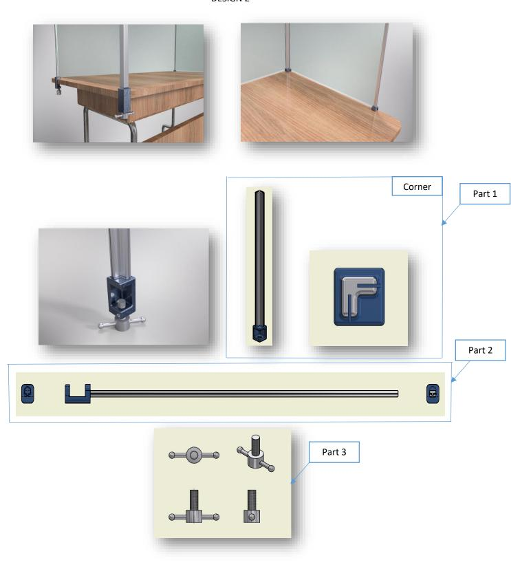
The above view is a description of application of the second Garry dispersing tool, there is a slight difference in design to the first because of the design of the second there is the addition of a new part of the part 1 that is pointless on the corner of each table, and in this design I make it more efficient because 1 table only requires part 1 = 2 pieces, Part 2 = 2 pieces and Part 3 = 4 pieces, and the components of these tools can be created using 3d printing to save more
